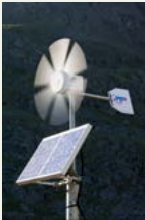
A solar electric panel and wind turbine being used to power a neon road sign.
