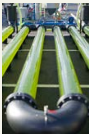
An AlgaeLink Algae growing system that is harvested to make ethanol and biodiesel, UK. Producing oil from algae in this way is much more efficient than from growing traditional plant oil crops like oil seed rape. It also has the benefit that it does not take up space that could be growing food crops.
